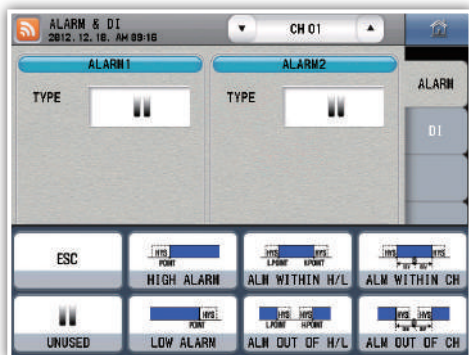
Fig. 45) Alarm selection screen
